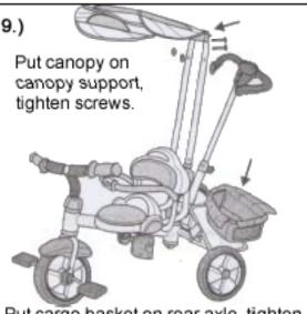
Put cargo basket on rear axle, tighten screws. Now it is ready to go!
