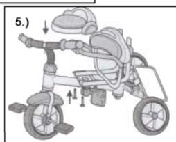
Place seat on seat support, tighten screws.
