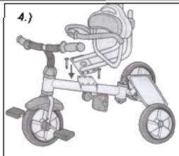
Place seat support on frame, tighten screws. Insert padded restraint bars onto seat support. Place seat back onto onto seat support. carefully tighten screws & avoid stripping the plastic.
